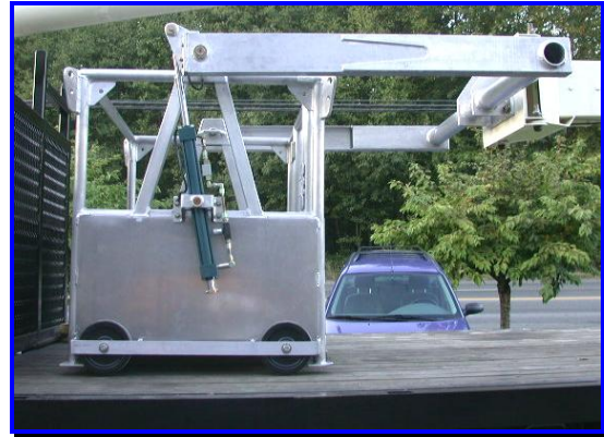
Platform Leveling System: Closed system brake locks the platform in place.
