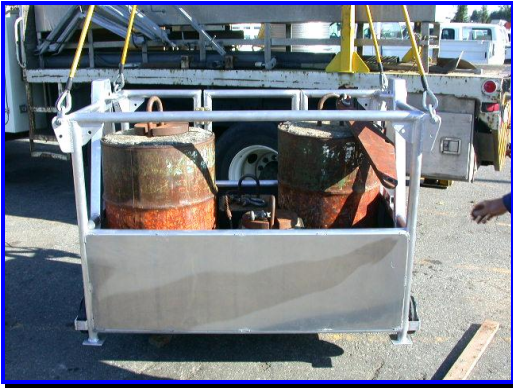
Aluminum Platform: Two man platform constructed of 6061-T6 aluminum which is rated at 600 lbs. and load tested at a 5:1 safety factor.
