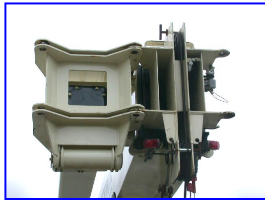
Sealed Boom: with desiccant cartridge reduces contamination, moisture and current leakage.
