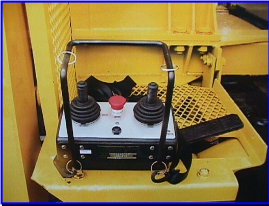
Personnel Platform Controls: Fully proportional adjustments for fine metering from the platform to ensure a safe and smooth entry into the limits of approach.
