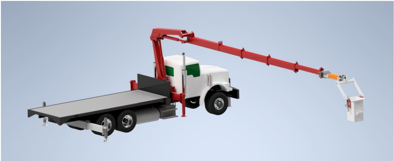
Above: Extended for personnel ingress/egress
