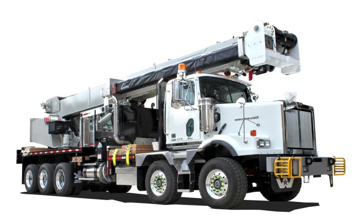
765kV Insulated Work Platform with 210° Hydraulic Articulation
