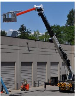
Left: Jib being tested at 575kV AC for the Cat. A certification. This jib achieves low current leakage reading due to its high dielectric strength and maintenance-free design. Low current leakage also improves worker comfort and safety.
